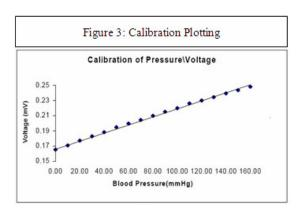
Calibration: clinical In measurements comparison of a new measurement technique with an old one is needed to see if they agree sufficiently for the new to replace the old. Blood pressure recorded by the pressure transducer was compared with pressure recorded using mercury sphygmomanometer (Aesculap, Nova-Presameter, Jetter and Scheerer, Germany) which is considered as gold standard for
