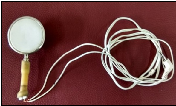
Figure-1: Constructed Electronic Stethoscope
